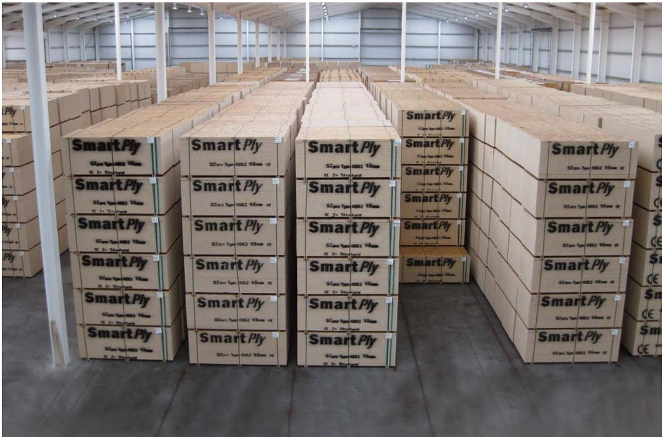
SmartPly OSB is manufactured from longitudinal timber strands measuring approximately 100mm in length x 40mm in width x 0.65mm in thickness. The strands are sliced from the logs in the direction of the grain to achieve maximum strength in the resulting panel.
